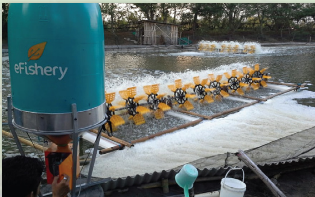
eFishery's automatic smart feeder uses sensors to detect hungry fish behavior and dispense the right amount of feed
